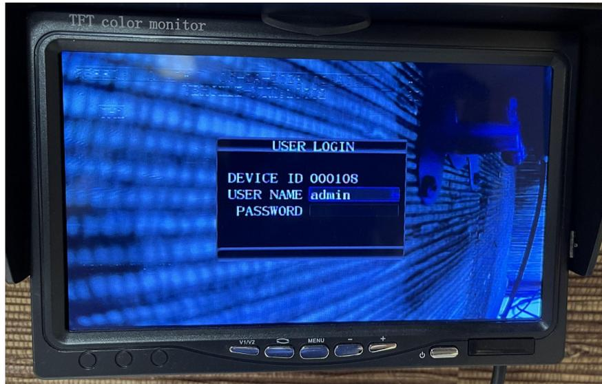
To log in to the menu, press the MENU button on the remote control. You will see the login screen come up. Place the cursor in the PASSWORD space and enter the admin password. The default password is SIX 8s (888888). Once the password is successfully entered, you will automatically be taken to the next screen.
